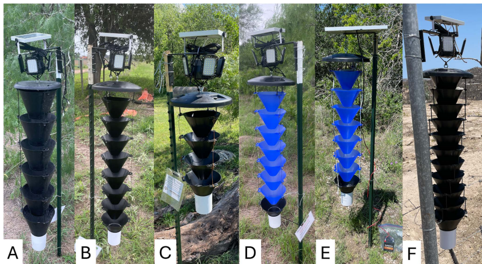
Fig 4. Five Kissing Bug Kill Trap prototypes evaluated in Texas in 2023. A) TRAP2A, Multitrap with 6 funnels and 4-panel lights; B) Lindgren black funnel trap with 8 funnels and 4-panel lights (TRAP4); C) Lindgren black funnel with 4 funnels and 4-panel light (TRAP5); D) Lindgren blue funnel trap with 8 funnels and 4-panel light; E) Lindgren blue funnel trap with 8 funnels and blue LED light strips (TRAP7); F) Lindgren black funnel nested together with 11 funnels and small LED (TRAP-MEXICO).
